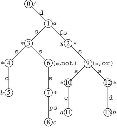
Figure 3:  $Q = /d :: a[c :: b \text{ and not ps :: c}] /fs :: *[c :: a \text{ or } d :: b]$
